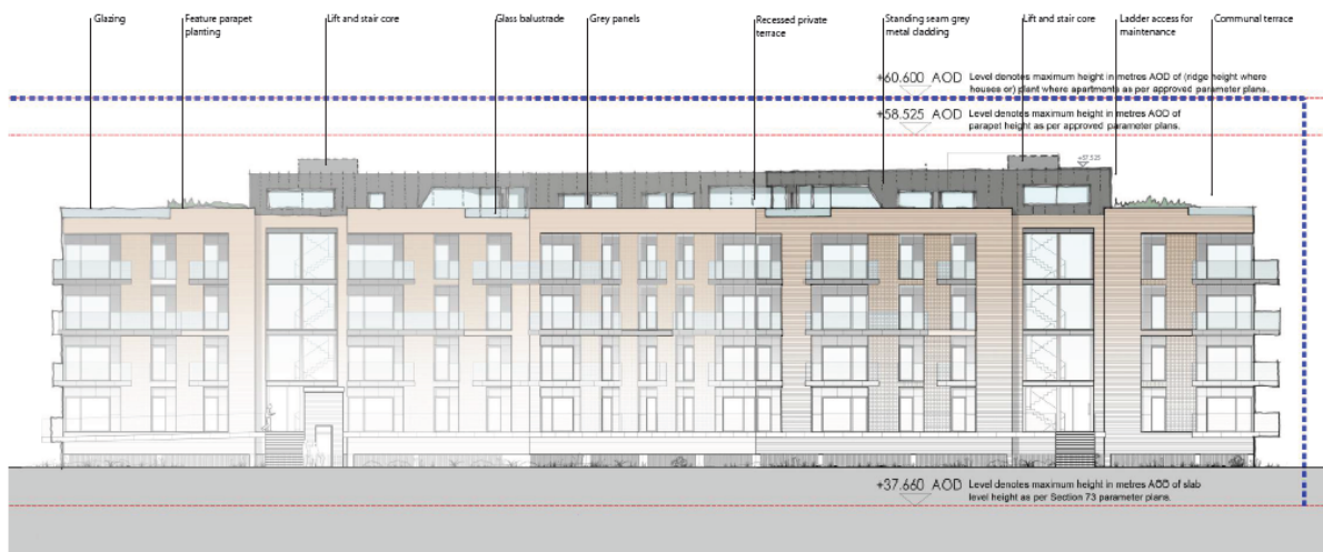
Figure 6: Street Elevation Block 5B
